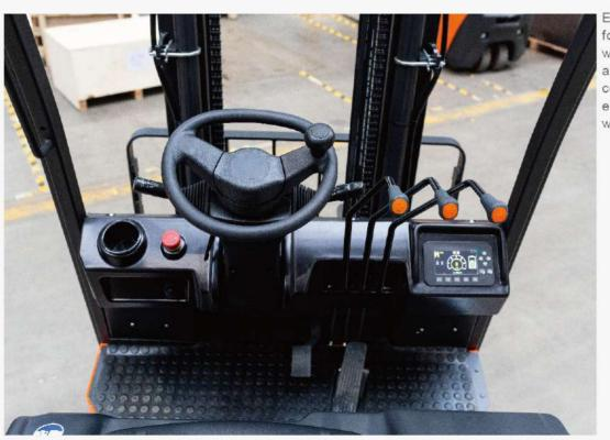
Ergonomics design for comfort operation with wide mast view and easy right-sided control levers and easy steering wheel with knob.
